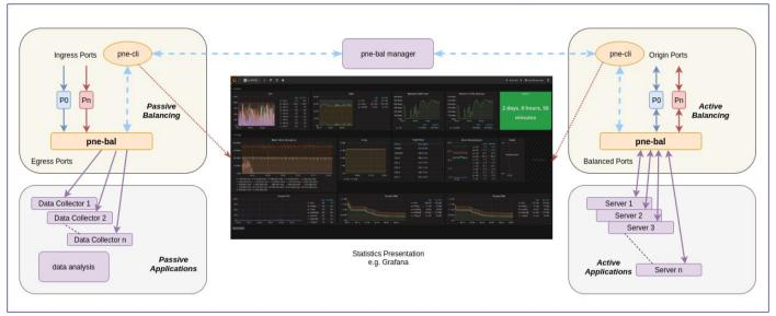
The pne-balancer distributes Ethernet frames received on ingress ports to egress ports in order to balance the traffic load over several egress ports. Balancing is based on bi-directional 2-tuple IP addresses or Round-Robin. Customized balancing criteria can be added. Both passive and active traffic is supported. An API allows for its integration into downstream consumers and management system.
