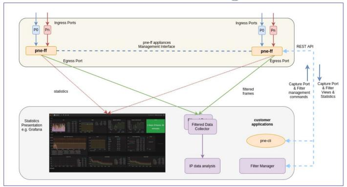
The pne-ff is a IP filtering appliance that operates in standalone mode or integrated into downstream systems. It offers many multi-speed links from a high port-density platform with a small footprint both in space and thermals. Its P4 programmable platform means that features can be quickly customized to particular needs. Resilient configurations are possible without duplicated hardware for two or more units.
